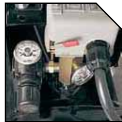
Regulator and two gauges for tank and outlet pressure
