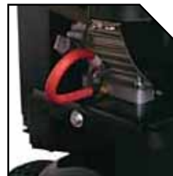
Belt tightening system pulls engine straight to ensure constant belt alignment
